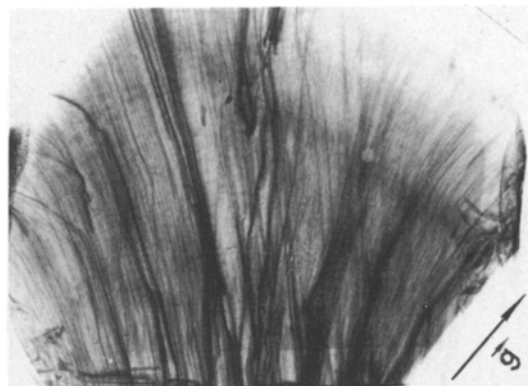
Figure 5 X-ray traverse topograph of the surface layer of synthetic fluorophlogopite crystal using Mo radiation and (060) reflection. There are many sub-grain boundaries and dislocations along the growth direction.
